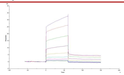
Human PSGL-1, His Tag (Cat. No. PS1-H52H9) immobilized on CM5 Chip can bind Human B7-H5, Fc Tag (Cat. No. B75-H5259) with an affinity constant of 0.213  $\mu$ M as determined in a SPR assay (Biacore T200) (Routinely tested).
