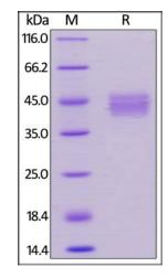
Human BCMA Protein, Llama IgG2b Fc Tag on SDS-PAGE under reducing (R) condition. The gel was stained with Coomassie Blue. The purity of the protein is greater than 90%.
