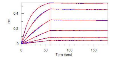
Loaded Siglec-3 MAb (Mouse IgG1) on AMC Biosensor, can bind Human Siglec-3, Fc Tag (Cat. No. CD3-H5257) with an affinity constant of 0.329 nM as determined in BLI assay (ForteBio Octet Red96e) (Routinely tested).
