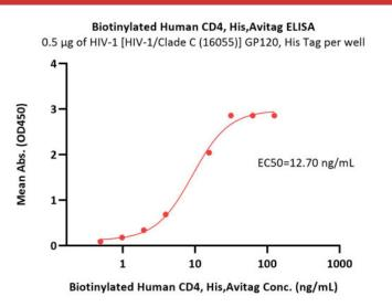
Immobilized Ibalizumab at 1  $\mu$ g/mL (100  $\mu$ L/well) can bind Biotinylated Human CD4, His,Avitag (Cat. No. CD4-H82E8) with a linear range of 0.2-3 ng/mL (QC tested).
