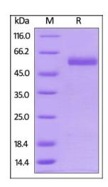
Biotinylated Human CD4, His, Avitag on SDS-PAGE under reducing (R) condition. The gel was stained overnight with Coomassie Blue. The purity of the protein is greater than 95%.
