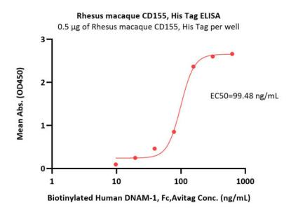
Immobilized Rhesus macaque CD155, His Tag (Cat. No. CD5-R52H5) at 5  $\mu$ g/mL (100  $\mu$ L/well) can bind Biotinylated Human DNAM-1, Fc,Avitag (Cat. No. DN1-H82F9) with a linear range of 10-156 ng/mL (Routinely tested).
