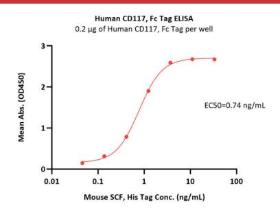
Immobilized Human CD117, Fc Tag (Cat. No. CD7-H5255) at 2  $\mu$ g/mL (100  $\mu$ L/well) can bind Mouse SCF, His Tag (Cat. No. SCF-M5228) with a linear range of 0.05-1 ng/mL (Routinely tested).
