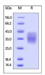
Biotinylated Human EMMPRIN, Avitag, His Tag on SDS-PAGE under reducing (R) condition. The gel was stained overnight with Coomassie Blue. The purity of the protein is greater than 92%.
