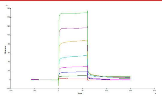
Biotinylated Human CD32a (R167), His, Avitag (Cat. No. CDA-H82E5) immobilized on SA Chip can bind Rituximab with an affinity constant of 0.802 μM as determined in a SPR assay (Biacore T200) (Routinely tested).
