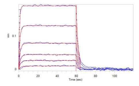
Loaded Human CD155, Fc Tag (Cat. No. CD5-H5251) on Protein A Biosensor, can bind Cynomolgus DNAM-1, His Tag (Cat. No. DN1-C52H9) with an affinity constant of 0.88  $\mu$ M as determined in BLI assay (ForteBio Octet Red96e) (Routinely tested).
