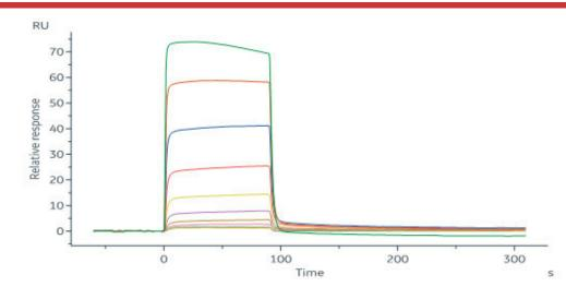
Human CD155, Fc Tag (Cat. No. CD5-H5251) captured on CM5 chip via Antihuman IgG Fc antibodies surface can bind Mouse DNAM-1, His Tag (Cat. No. DN1-M52H5) with an affinity constant of 0.816  $\mu$ M as determined in a SPR assay (Biacore 8K) (QC tested).
