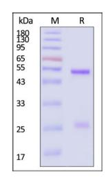
Biotinylated Human IgG1 (N297A) Kappa Isotype Control (mAb) on SDS-PAGE under reducing (R) condition. The gel was stained with Coomassie Blue. The purity of the protein is greater than 90% (With <u>Star Ribbon Pre-stained Protein Marker</u>).
