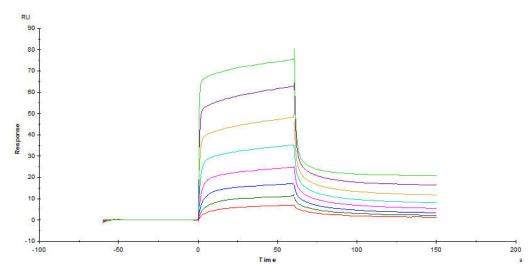
Captured Biotinylated Cynomolgus / Rhesus macaque FcRn Heterodimer Protein, His,Avitag&Strep II Tag (Cat. No. FCM-C82W5) on Biotin CAP - Series S sensor Chip can bind Herceptin® with an affinity constant of 0.241  $\mu$ M as determined in a SPR assay (Biacore T200) (QC tested).
