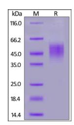
Mouse FGFR2 (IIIb), His Tag on SDS-PAGE under reducing (R) condition. The gel was stained with Coomassie Blue. The purity of the protein is greater than 90%.
