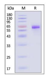
Mouse FOLR1 Protein, Fc Tag on SDS-PAGE under reducing (R) condition. The gel was stained with Coomassie Blue. The purity of the protein is greater than 90% (With Star Ribbon Pre-stained Protein Marker).
