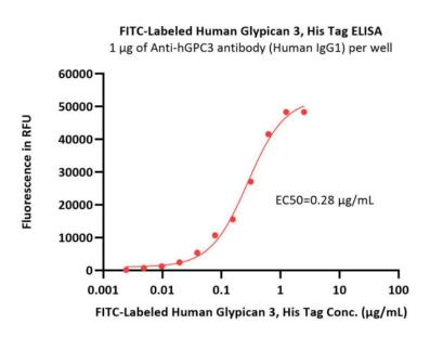
Immobilized Anti-hGPC3 antibody (Human IgG1) at 10  $\mu$ g/mL (100  $\mu$ L/well) can bind FITC-Labeled Human Glypican 3, His Tag (Cat. No. GP3-HF2H1) with a linear range of 0.078-0.625  $\mu$ g/mL (QC tested).
