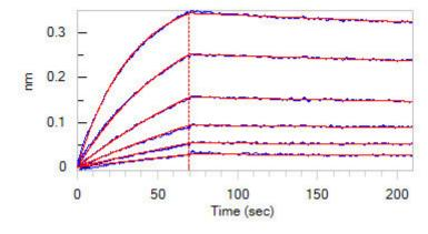
Loaded Hercecptin on AHC Biosensor, can bind Human Her2, Tag Free (Cat. No. HE2-H5212) with an affinity constant of 1.45 nM as determined in BLI assay (ForteBio Octet Red96e) (Routinely tested).
