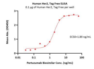
Immobilized Human Her2, Tag Free (Cat. No. HE2-H5212) at 1  $\mu$ g/mL (100  $\mu$ L/well) can bind Pertuzumab Biosimilar with a linear range of 0.1-4  $\mu$ g/mL (Routinely tested).
