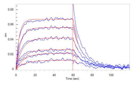
Loaded Human HVEM, Fc Tag (Cat. No. HVM-H5258) on Protein A Biosensor, can bind Human CD160, His Tag (Cat. No. BY5-H5229) with an affinity constant of 0.44  $\mu$ M as determined in BLI assay (ForteBio Octet Red96e) (Routinely tested).
