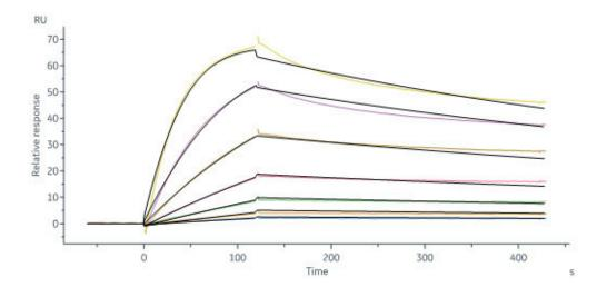
Monoclonal Anti-IFNγ antibody, Mouse IgG2a (8C5F8) (Cat. No. IFN-S120) captured on CM5 chip via anti-mouse antibodies surface can bind Human IFN-gamma, premium grade (Cat. No. IFG-H4211) with an affinity constant of 0.933 nM as determined in a SPR assay (Biacore 8K) (Routinely tested).
