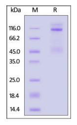
Rat IGF-I R, His Tag on SDS-PAGE under reducing (R) condition. The gel was stained with Coomassie Blue. The purity of the protein is greater than 90%.
