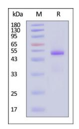
Mouse IL-11 Protein, Fc Tag on SDS-PAGE under reducing (R) condition. The gel was stained with Coomassie Blue. The purity of the protein is greater than 90% (With Star Ribbon Pre-stained Protein Marker).
