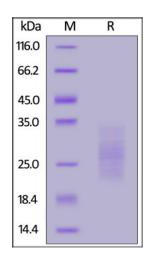
Biotinylated Mouse IL-31, His, Avitag on SDS-PAGE under reducing (R) condition. The gel was stained with Coomassie Blue. The purity of the protein is greater than 90%.
