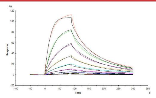
Anti-IL-3 R alpha Antibody, Human IgG1 immobilized on CM5 Chip can bind Human IL-3 R alpha, Fc Tag (Cat. No. ILA-H5252) with an affinity constant of 50.3 nM as determined in a SPR assay (Biacore T200) (QC tested).
