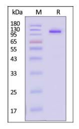
Cynomolgus IL-12 R beta 1 Protein, Fc Tag on SDS-PAGE under reducing (R) condition. The gel was stained with Coomassie Blue. The purity of the protein is greater than 95% (With <u>Star Ribbon Pre-stained Protein Marker</u>).
