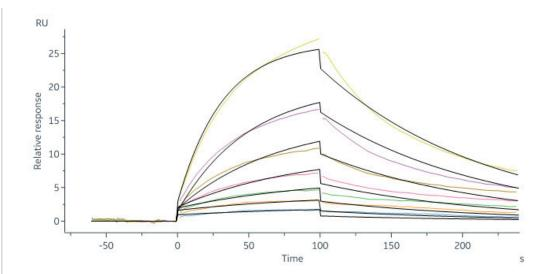
Human IL-17 RA, Fc Tag captured on CM5 chip via Anti-human IgG Fc antibodies surface can bind Mouse IL-17F, His Tag (Cat. No. ILF-M5249) with an affinity constant of 2.99  $\mu$ M as determined in a SPR assay (Biacore 8K) (Routinely tested).
