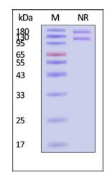
Human ITGA5&ITGB1 Heterodimer Protein, Tag Free&Tag Free on SDS-PAGE under non-reducing (NR) condition. The gel was stained with Coomassie Blue. The purity of the protein is greater than 95% (With <u>Star</u> <u>Ribbon Pre-stained Protein Marker</u>).
