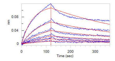
Loaded Human Laminin 121 Protein, premium grade (Cat. No. LA1-H5261) on Protein A Biosensor, can bind Human ITGA7X2B&ITGB1 Heterodimer Protein, His Tag&Tag Free (Cat. No. IT1-H52W8) with an affinity constant of 6.23 nM as determined in BLI assay (ForteBio Octet Red96e) (QC tested).
