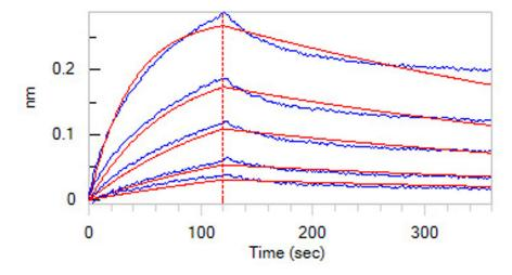
Loaded Human Laminin 121 Protein, premium grade (Cat. No. LA1-H5261) on Protein A Biosensor, can bind Human ITGA7X2B&ITGB1 Heterodimer Protein, His Tag&Tag Free (Cat. No. IT1-H52W8) with an affinity constant of 6.95 nM as determined in BLI assay (ForteBio Octet Red96e) (Routinely tested).
