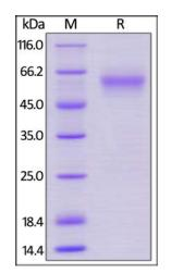
Mouse LAIR1 Protein, Mouse IgG2a Fc Tag on SDS-PAGE under reducing (R) condition. The gel was stained with Coomassie Blue. The purity of the protein is greater than 95%.
