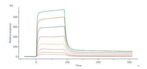
Human MCAM, His Tag (Cat. No. CD6-H5229) immobilized on CM5 Chip can bind Human Laminin 411 Protein, premium grade (Cat. No. LAT-H5263) with an affinity constant of 0.115  $\mu$ M as determined in a SPR assay (Biacore 8K) (Routinely tested).
