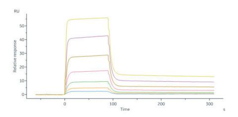
Human MCAM, His Tag (Cat. No. CD6-H5229) captured on CM5 chip via anti-His antibody can bind Human Laminin 411 Protein, premium grade (Cat. No. LAT-H5263) with an affinity constant of 27.9 nM as determined in a SPR assay (Biacore 8K) (Routinely tested).
