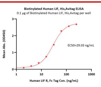
Immobilized Biotinylated Human LIF, His,Avitag (Cat. No. LIF-H82E2) on SA-coated surface at 1  $\mu$ g/mL (100  $\mu$ L/well) can bind Human LIF R, Fc Tag (Cat. No. LIR-H4252) with a linear range of 1-31 ng/mL (QC tested).
