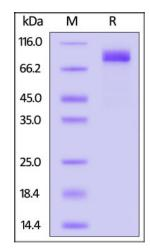
Biotinylated Human Nectin-3, Fc, Avitag on SDS-PAGE under reducing (R) condition. The gel was stained with Coomassie Blue. The purity of the protein is greater than 95%.
