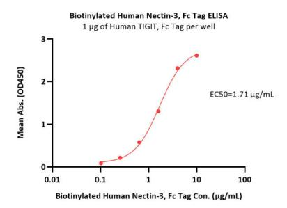
Immobilized Human TIGIT, Fc Tag (Cat. No. TIT-H5254) at 10  $\mu$ g/mL (100  $\mu$ L/well) can bind Biotinylated Human Nectin-3, Fc,Avitag (Cat. No. PV3-H82F3) with a linear range of 0.102-4  $\mu$ g/mL (Routinely tested).
