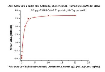
Immobilized SARS-CoV-2 S1 protein, His Tag (Cat. No. S1N-C52H2) at 2  $\mu$ g/mL (100  $\mu$ L/well) can bind Anti-SARS-CoV-2 Spike RBD Antibody, Chimeric mAb, Human IgG1 (AM130) (Cat. No. S1N-M13A1) with a linear range of 0.078-1.25 ng/mL (QC tested).
