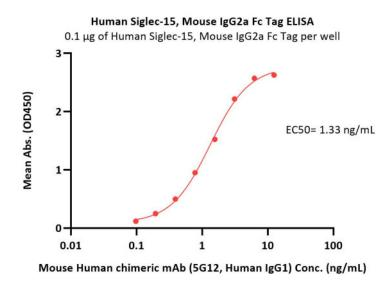
Immobilized Human Siglec-15, Mouse IgG2a Fc Tag (Cat. No. SG5-H5254) at 1  $\mu$ g/mL (100  $\mu$ L/well) can bind Mouse Human chimeric mAb (5G12, Human IgG1) with a linear range of 0.1-2 ng/mL (Routinely tested).
