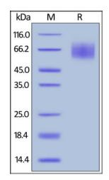
Mouse SIRP alpha, His Tag on SDS-PAGE under reducing (R) condition. The gel was stained with Coomassie Blue. The purity of the protein is greater than 95%.
