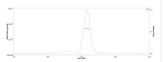
The purity of Mouse SIRP alpha, His Tag (Cat. No. SIA-M52H4) is more than 90% and the molecular weight of this protein is around 50-70 kDa verified by SEC-MALS.
