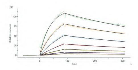
Biotinylated Human Sortilin Protein, His, Avitag (Cat. No. SON-H82E9) captured on Biotin CAP-Series S Sensor Chip can bind Human Progranulin Protein, His Tag (Cat. No. PGN-H52H3) with an affinity constant of 0.355 μM as determined in a SPR assay (Biacore 8K) (QC tested).
