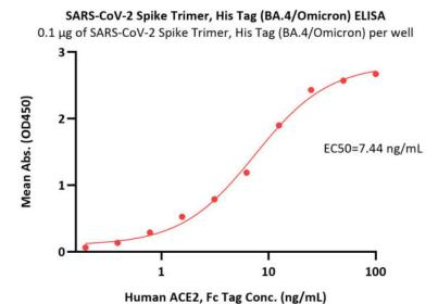
Immobilized SARS-CoV-2 Spike Trimer, His Tag (BA.4/Omicron) (Cat. No. SPN-C5229) at 1  $\mu$ g/mL (100  $\mu$ L/well) can bind Human ACE2, Fc Tag (Cat. No. AC2-H5257) with a linear range of 0.2-13 ng/mL (QC tested).
