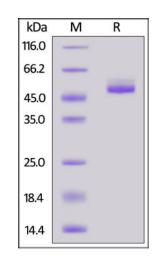
Cynomolgus / Rhesus macaque TIGIT, Mouse IgG2a Fc Tag on SDS-PAGE under reducing (R) condition. The gel was stained with Coomassie Blue. The purity of the protein is greater than 90%.
