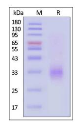
Human TNFR1, His Tag on SDS-PAGE under reducing (R) condition. The gel was stained with Coomassie Blue. The purity of the protein is greater than 90% (With <u>Star Ribbon Pre-stained Protein Marker</u>).
