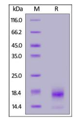
Human TSPAN8, His Tag on SDS-PAGE under reducing (R) condition. The gel was stained with Coomassie Blue. The purity of the protein is greater than 90%.
