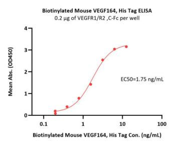
Immobilized VEGFR1/R2 ,C-Fc at 2  $\mu$ g/mL (100  $\mu$ L/well) can bind Biotinylated Mouse VEGF164, His,Avitag (Cat. No. VE4-M82Q3) with a linear range of 0.1-3 ng/mL (QC tested).
